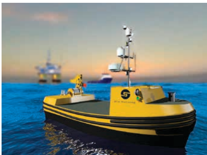
Figure 1. The autonomous work boat is Sea Machine's first production hull. While primarily designed for heavy work such as towing and barge moving, the V1 also has the capability for extended survey operations and station keeping/standoff applications.
