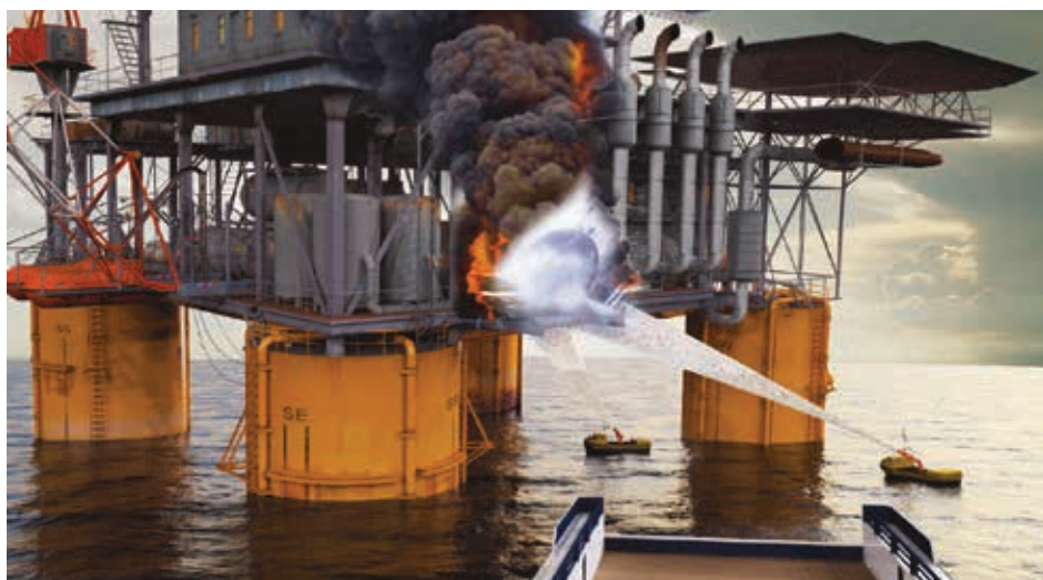
Figure 4. The Sea Machines V1 makes an ideal small fire boat, allowing the vehicle to get closer to, or under hazardous fires than would normally be safe with operators aboard. The V1’s accurate stand off and station keeping capabilities will keep the vehicle where the operators set it, while allowing them direct control of the fire pump.
